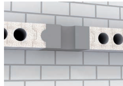
Porous concrete ceiling (possibly with cavities)
