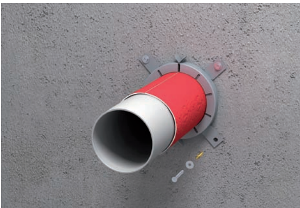
Plugging the retaining tab with the jointly supplied fixing set (as an option the tabs can also be bent through 90° and bedded in mortar!)
